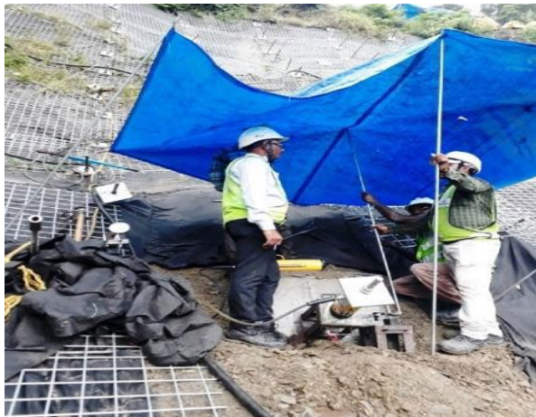
Pull-out Test on the steel nailing of existing valley slope
