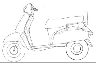
The rider can step through to mount the vehicle having platform/floorboard, and foot rests for the rider are integral with platform/footboard
