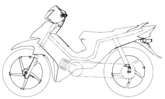
For mounting the vehicle, the rider can step through the low structure and rider's foot rests are mounted on chassis/engine
