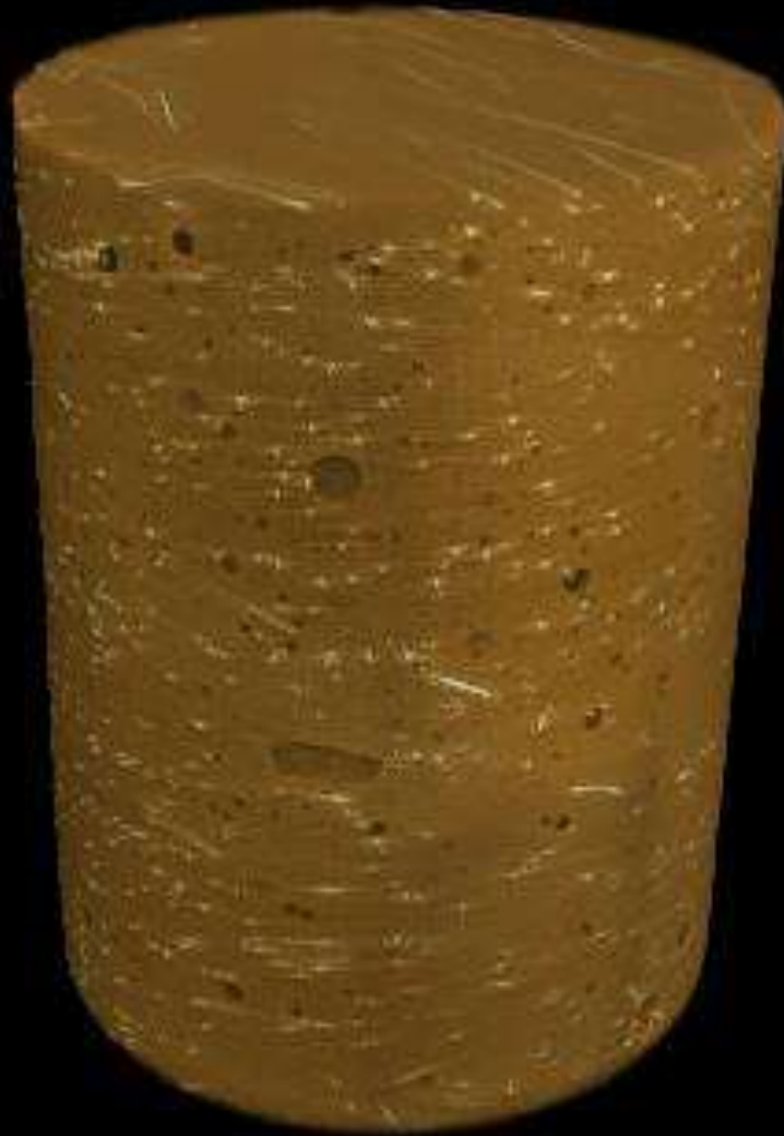
CT Scan on core sample
